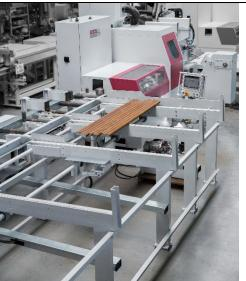
Round bars and pipes are usually delivered in a bundle and placed on the robust material storage of the magazine. There, the bundle is opened and the rods are distributed as a layer on the magazine.
