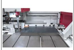
The combination of NC-controlled positioning unit and intelligent control allows plates to be split in an automated manner.
