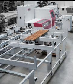
Round bars and pipes are usually delivered in a bundle and placed on the robust material storage of the magazine. There, the bundle is opened and the rods are distributed as a layer on the magazine.
