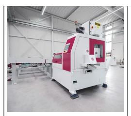
The HCS 150 E high speed circular saw is the basis for mass production with the highest output and quality. It cuts solid materials and tubes up to 152.4 mm (6 in.) in diameter or square material up to 130 x 130 mm edge dimensions.
